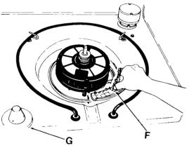
The coarse strainer may be removed, if necessary, without removing the other filters. TO REMOVE, lift strainer out by squeezing center section (F) and remove. TO REPLACE, squeeze center section so clips snap into square notch.
