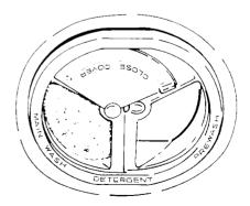
Fill the Main Wash compartment for the Light / China Wash Cycle when the dinnerware is lightly soiled.
